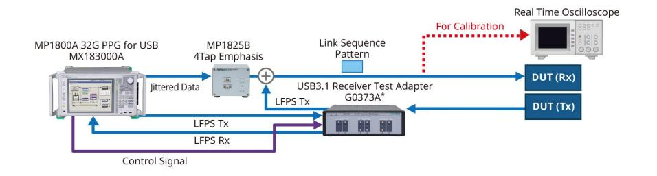
USB 3.1 Measurement Set-up
